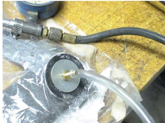
No-Leak(tm) vacuum bag fitting
