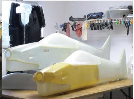
First two fuselages out of the molds
