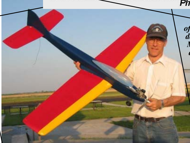
MOM #2 Rich Boelts displayed his latest nitro burner, a refurbished Dirty Birdy, reportedly built 25 to 30 years ago by Carlos Cartagena. Rich removed the original silk and dope covering and re-covered with blue, red and yellow monokote. Using a Hitec radio system and an O.S. 52 four stroke, this part of RC history will make its return to competition in this seasons pattern contests.
